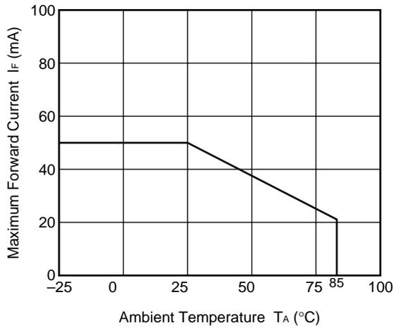
MAXIMUM LOAD CURRENT vs. AMBIENT TEMPERATURE
