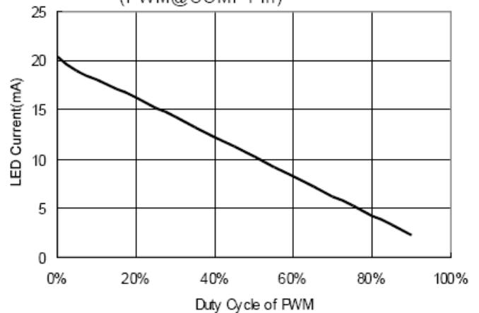
**Typical Performance Characteristics** (cont.) (@ $T_A = +25^\circ\text{C}$ ,  $V_{DD} = 5\text{V}$ , unless otherwise specified.)
