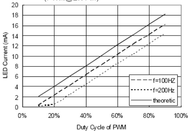
12. LED Current VS Duty Cycle of PWM
