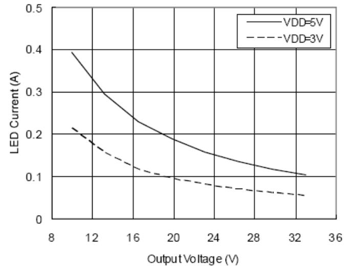
**Typical Performance Characteristics** (cont.) (@ $T_A = +25^\circ\text{C}$ ,  $V_{DD} = 5\text{V}$ , unless otherwise specified.)
