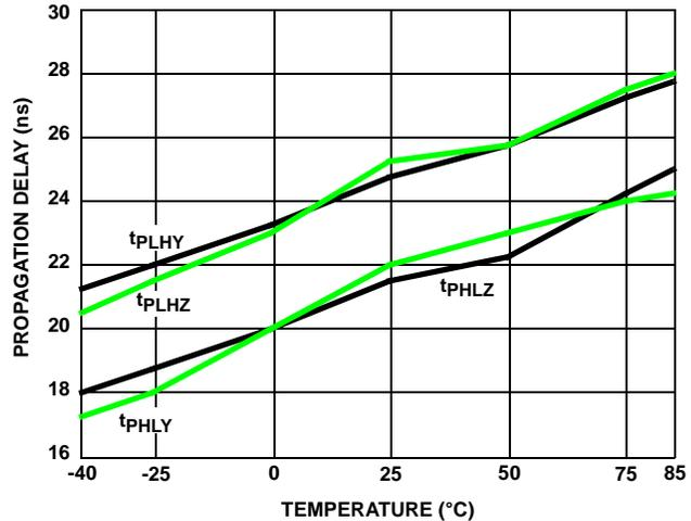
FIGURE 12. DRIVER PROPAGATION DELAY vs TEMPERATURE (ISL8490E/ISL8491E)
