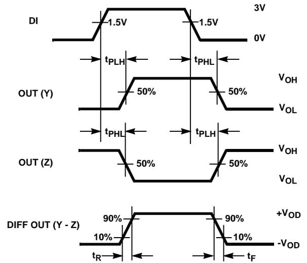
$$\text{SKEW} = |t_{PLH}(\text{Y or Z}) - t_{PHL}(\text{Z or Y})|$$
