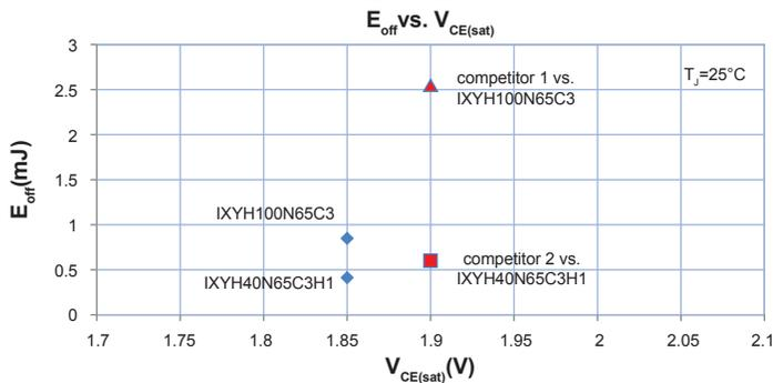
These 650V XPT™ IGBTs are designed to achieve an optimal balance between the turn-off energy loss and on-stage voltage, especially in hard-switching applications. The graph demonstrates a superior trade-off of the new IGBTs (in particular, the IXYH100N65C3 against competitor 1 and IXYH40N65C3H1 against competitor 2).
