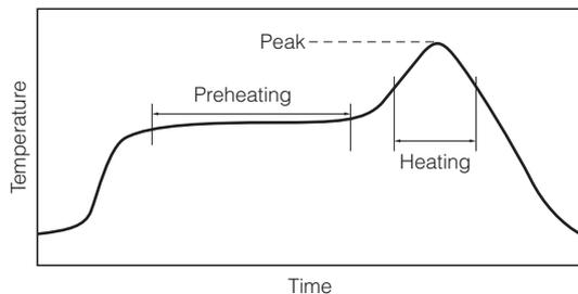
For soldering (Example : Sn/Pb)
