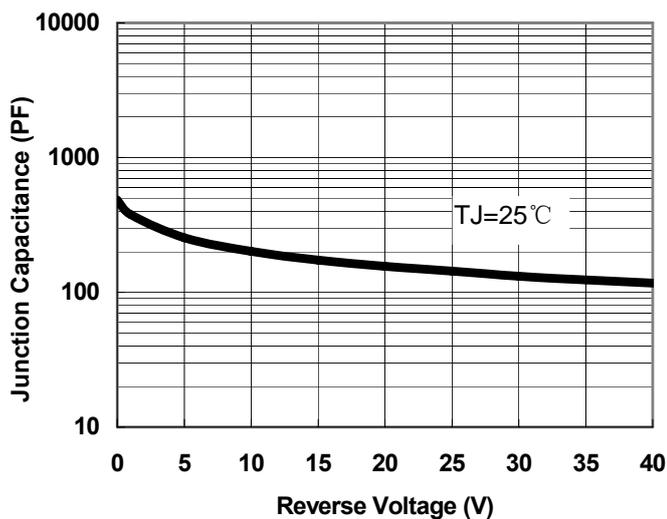
Fig.1-Typical Junction Capacitance
