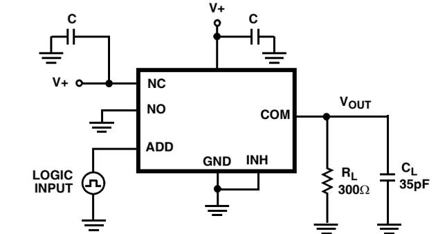
Repeat test for other switches.  $C_L$  includes fixture and stray capacitance.
