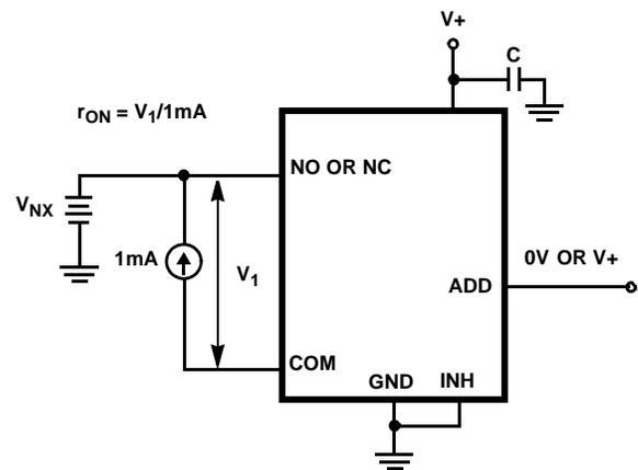
FIGURE 5.  $r_{ON}$  TEST CIRCUIT
