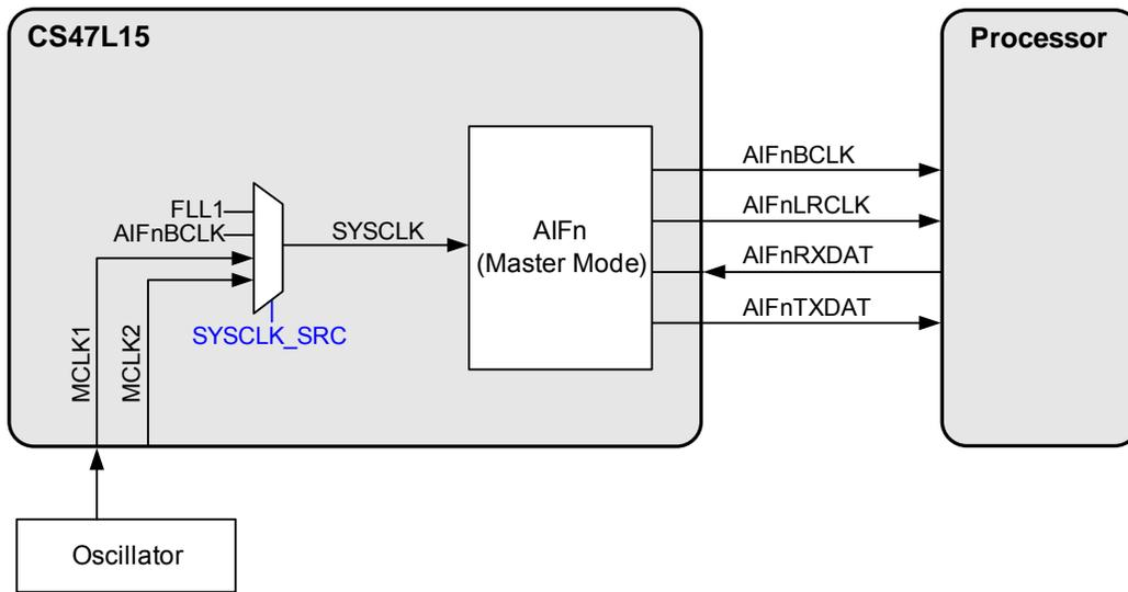
**Figure 5-13. AIF Master Mode, Using MCLK as Reference**
