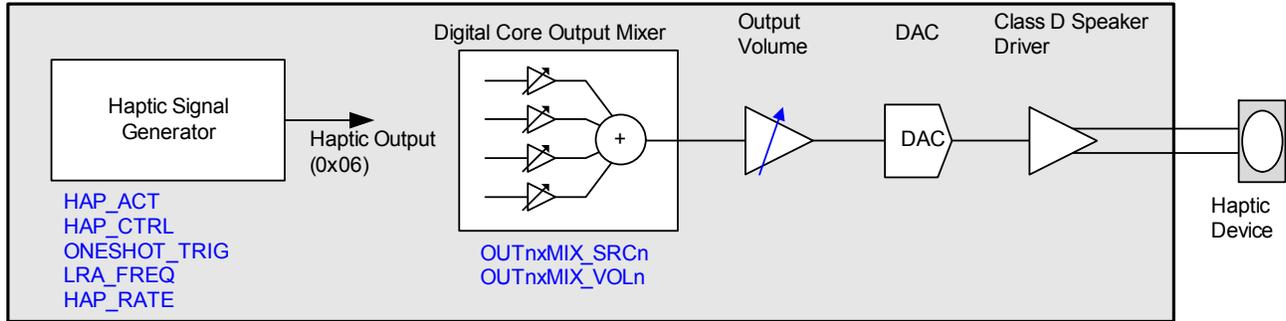
**Figure 4-26. Digital-Core Haptic Signal Generator**
