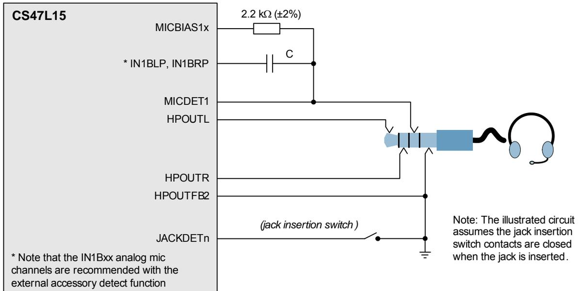
**Figure 4-55. Jack Detect and External Accessory Connections**
