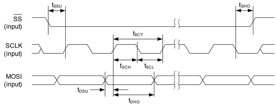
**2. Control interface timing—SPI Mode (read cycle)**
