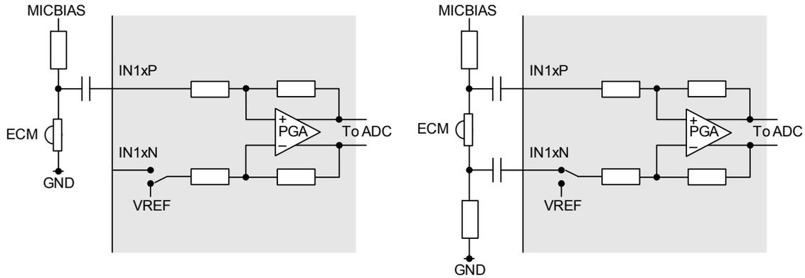
**Figure 5-2. Single-Ended and Differential ECM Microphone Connections**
