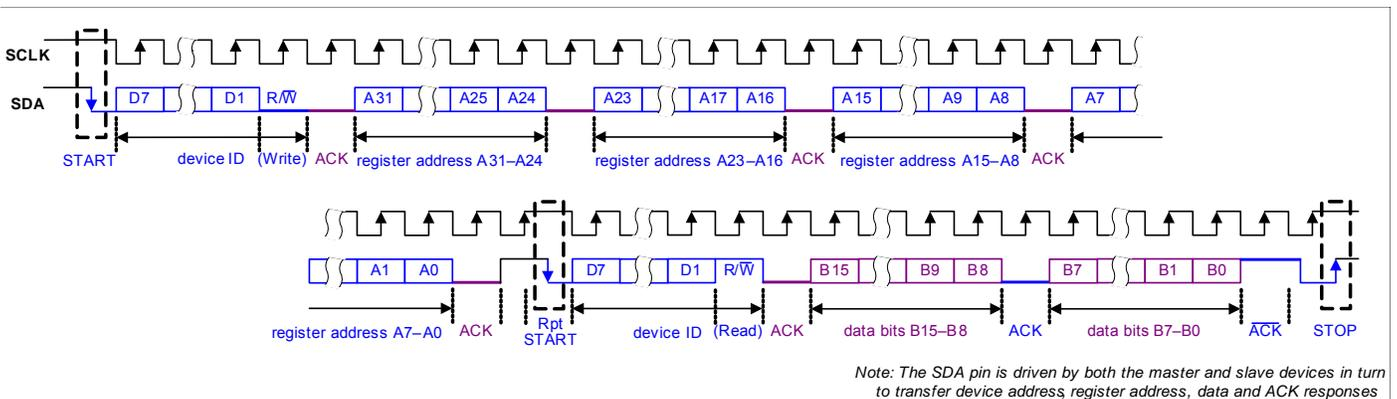
**Figure 4-73. Control Interface I<sup>2</sup>C Register Read (16-Bit Data Words)**
