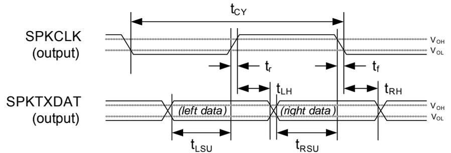
**2. Digital speaker (PDM) interface timing—Mode B**
