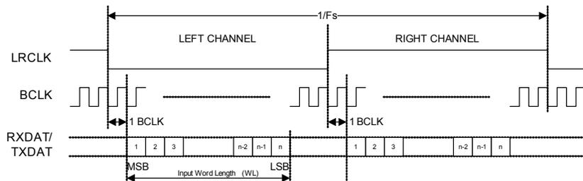
**Figure 4-38. I<sup>2</sup>S Data Format (Assuming n-Bit Word Length)**
