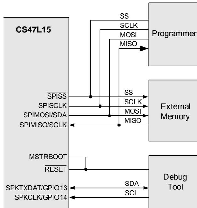
**Figure 4-78. SPI Master-Boot Connections**
