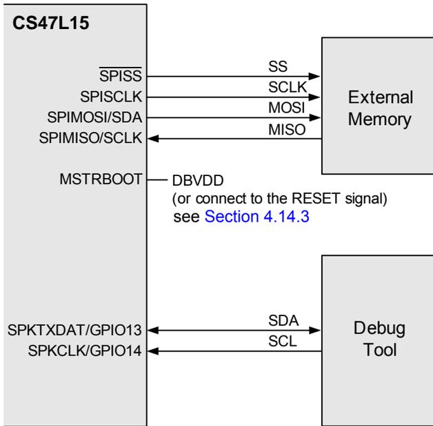
**Figure 4-69. I2C Slave and SPI Master Interfaces**
