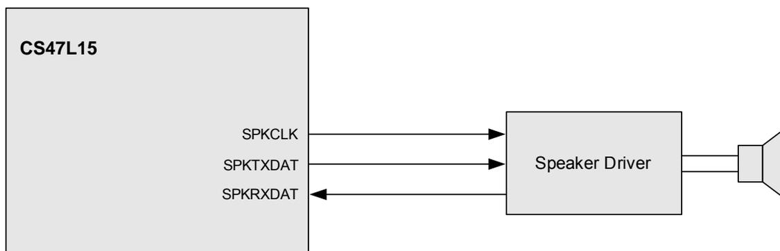
**Figure 4-54. Digital Speaker (PDM) Connection with Feedback**
