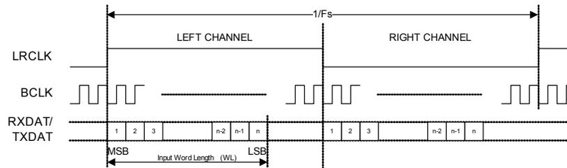
**Figure 4-39. Left-Justified Data Format (Assuming n-Bit Word Length)**
