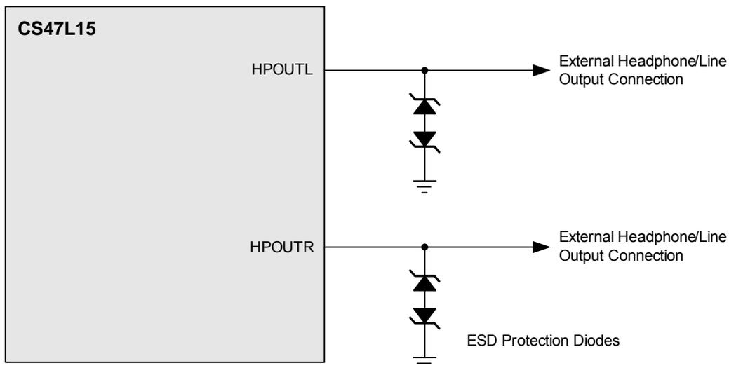
**Figure 5-6. ESD Diode Configuration for External Output Connections**
