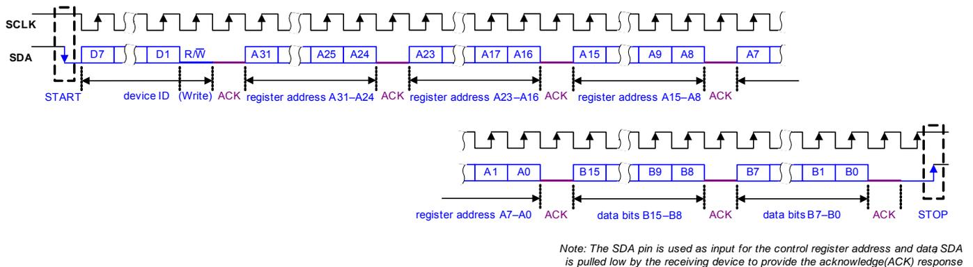
**Figure 4-72. Control Interface I<sup>2</sup>C Register Write (16-Bit Data Words)**
