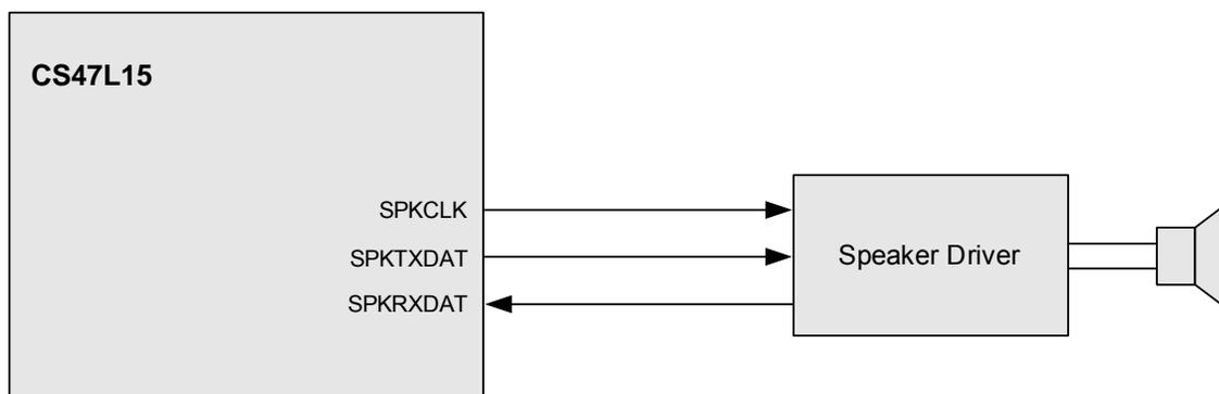
**Figure 4-13. Digital Speaker (PDM) Connection with Feedback**
