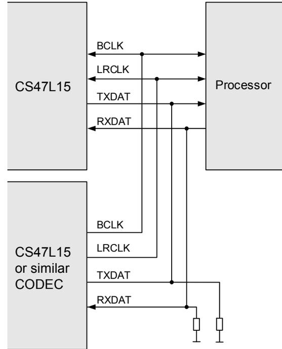
**Figure 4-45. TDM with Other Codec as Master**
