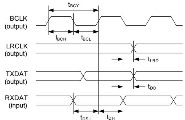
2. The timing of the AIF $n$ LRCLK signal is selectable. If the LRCLK advance option is enabled, the LRCLK transition is timed relative to the preceding BCLK edge. Under the required condition that BCLK is inverted in this case, the LRCLK transition is still timed relative to the falling BCLK edge.
