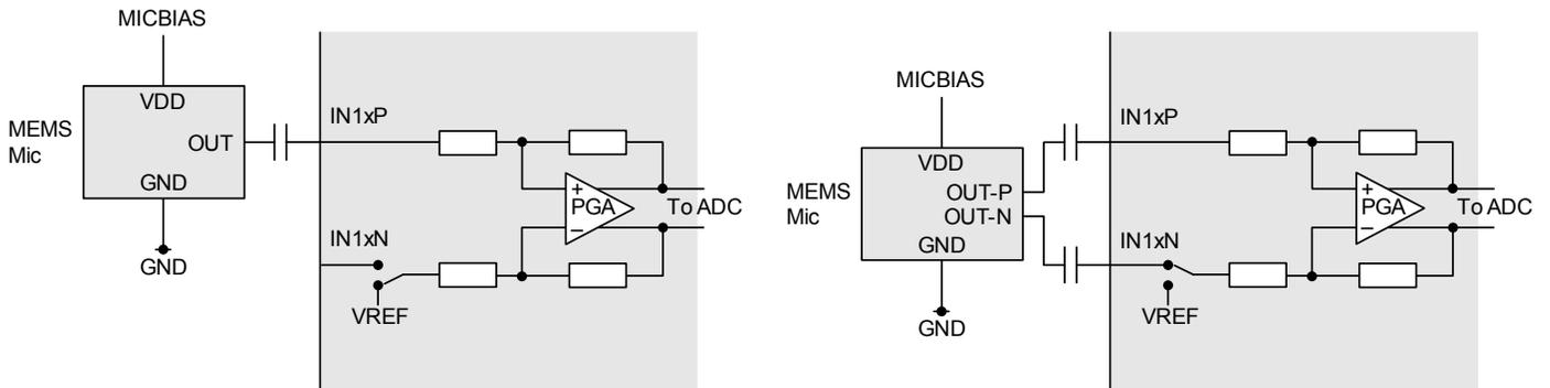
**Figure 5-3. Single-Ended and Differential Analog MEMS Microphone Connections**
