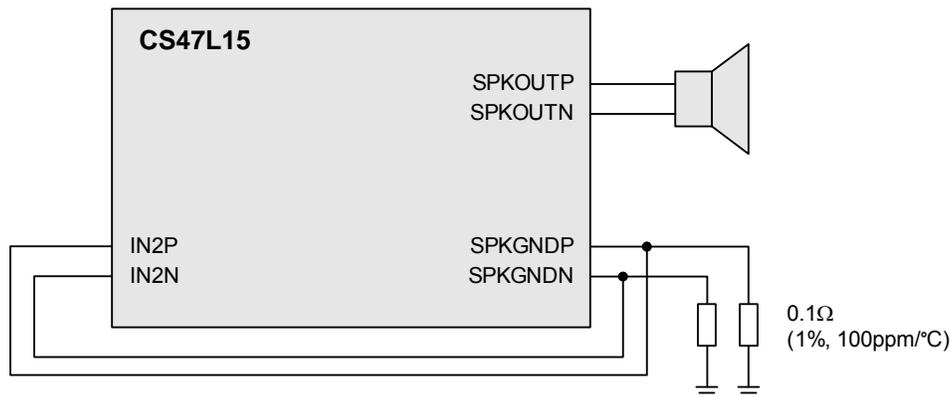
**Figure 5-10. Speaker Output Current Monitoring Connections (Speaker Protection)**
