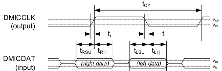
2. If the SPKRXDAT pin is configured for digital input, the SPKRXDAT timing requirements (with respect to SPKCLK) are the same as the DMICDAT timing requirements (with respect to DMICCLK).
