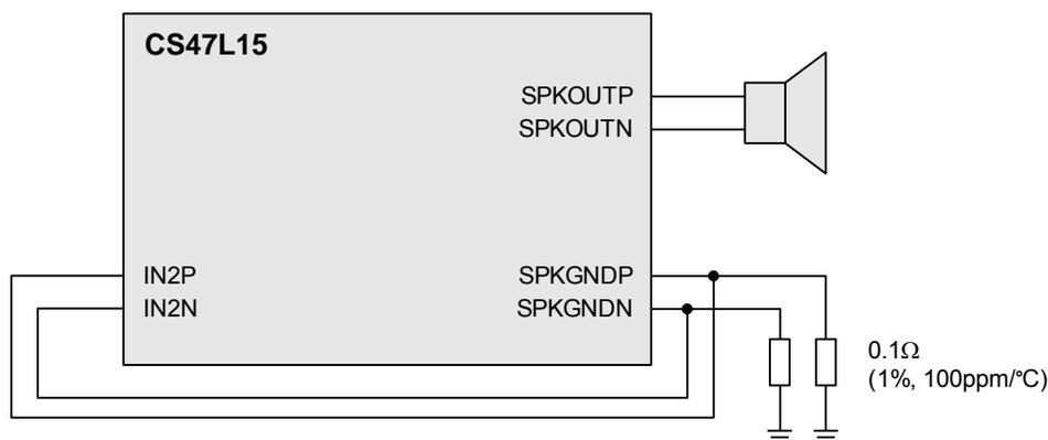
**Figure 4-51. Speaker Output Current Monitoring Connections (Speaker Protection)**
