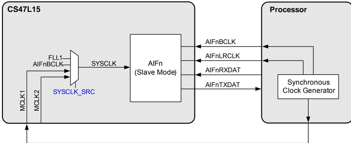
**Figure 5-17. AIF Slave Mode, Using MCLK as Reference**
