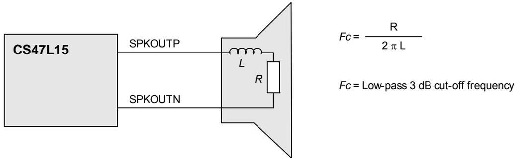
**Figure 5-9. Speaker Equivalent Circuit for Filterless Operation**
