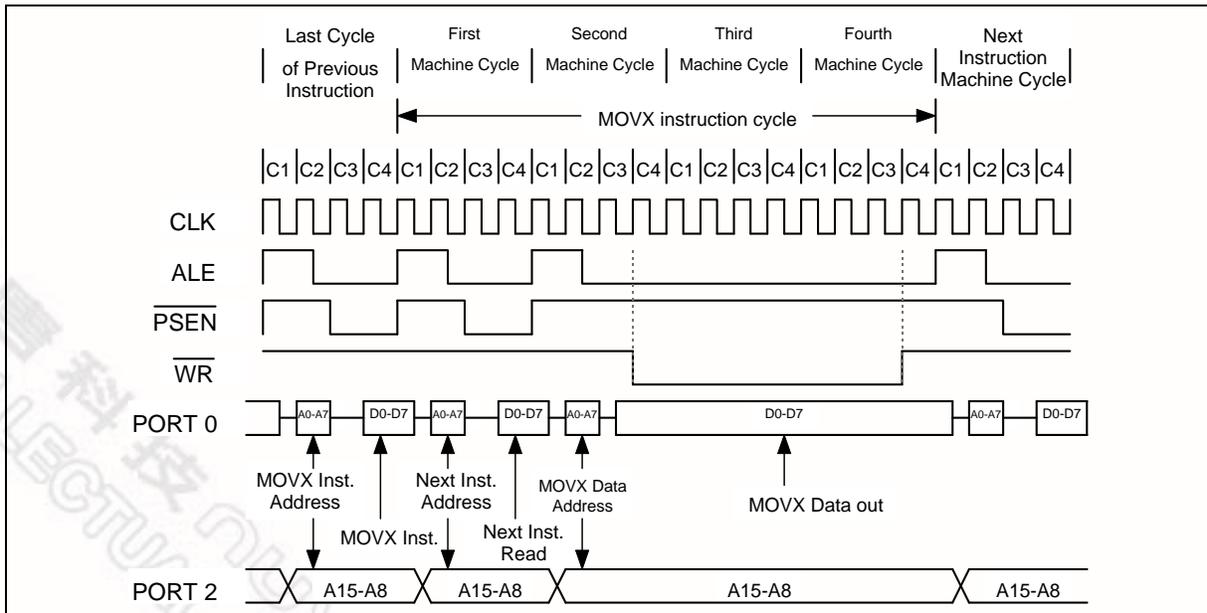
Figure 7-8 Data Memory Write with Stretch Value = 2
