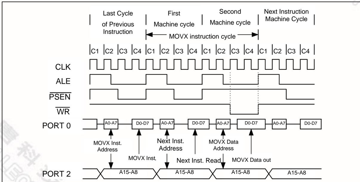
Figure 7-6 Data Memory Write with Stretch Value = 0
