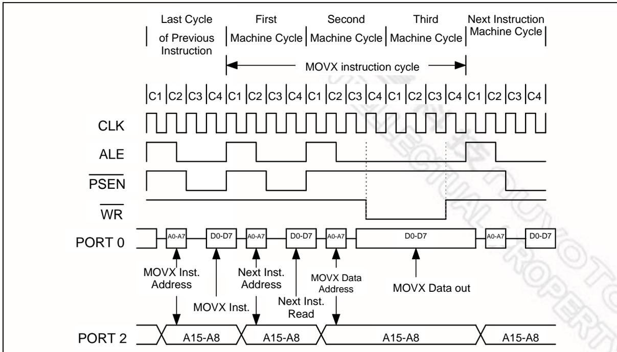
Figure 7-7 Data Memory Write with Stretch Value = 1
