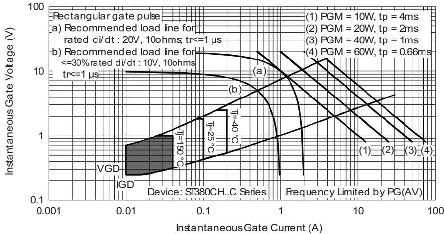
Fig. 11 - Gate Characteristics
