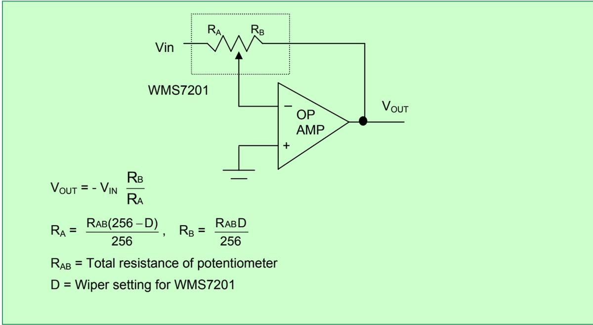
FIGURE 8 – PROGRAMMABLE INVERTING GAIN AMPLIFIER USING THE WMS7201
