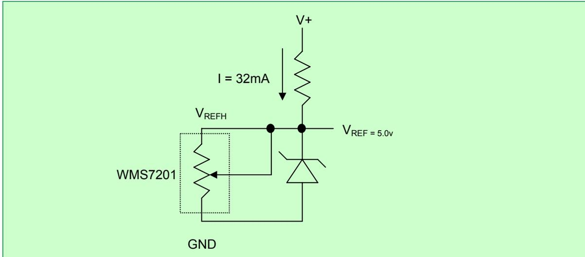
FIGURE 10 – WMS7201 TRIMMING VOLTAGE REFERENCE
