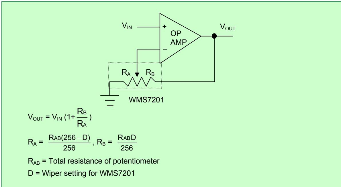
FIGURE 9 – PROGRAMMABLE NON-INVERTING GAIN AMPLIFIER USING THE WMS7201
