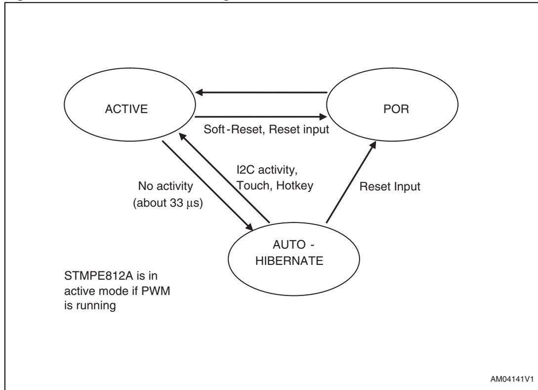
On power up reset, device goes to active state. However, as all the functional blocks are clocked off by default, no touch/hotkey activity is possible. If there are no I<sup>2</sup>C activities, device goes into auto-hibernate mode automatically.
