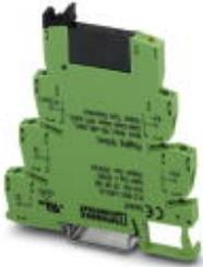
PLC-INTERFACE, consisting of PLC-BSC.../21 basic terminal block with screw connection and plug-in miniature solid-state relay, for mounting on DIN rail NS 35/7,5, 1 N/O contact, input: 120 V AC/110 V DC, output: 3 - 48 V DC/100 mA
