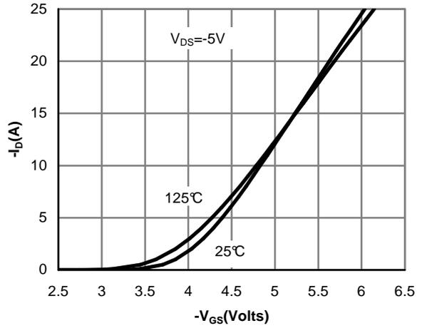
Figure 2: Transfer Characteristics
