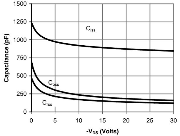
Figure 8: Capacitance Characteristics
