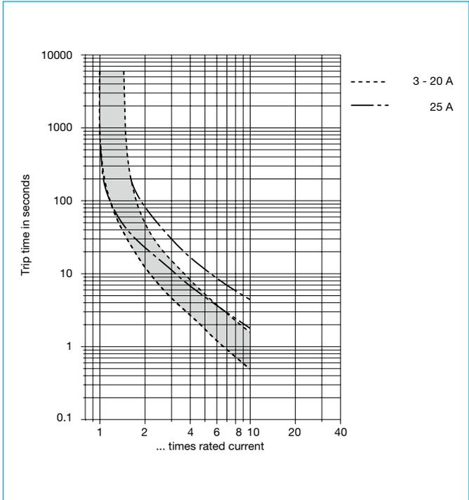
The time/current characteristic curve depends on the ambient temperature prevailing. In order to eliminate nuisance tripping, please multiply the circuit breaker current ratings by the derating factor shown below. See also section Technical information.
