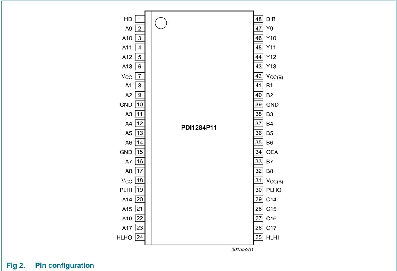
Fig 2. Pin configuration
