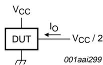
$I_O$  is measured by forcing  $0.5V_{CC}$  on the output. The output impedance can then be calculated as  $R_o = 0.5V_{CC} / |I_O|$ .
