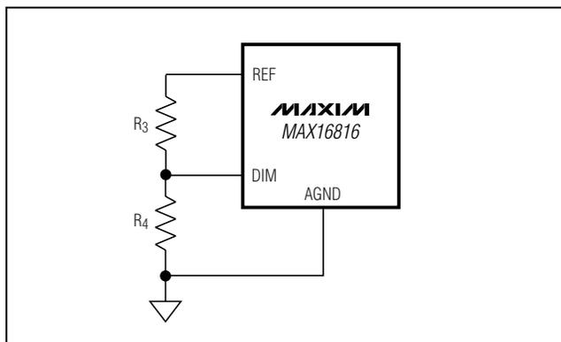
Figure 2. Creating DIM Input Signal from REF
