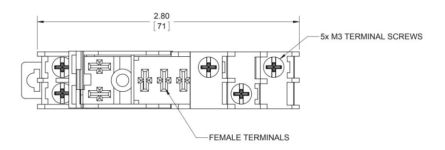
Tolerances: ± 0.02 in / 0.5 mm. All dimensions are in: inches [millimeters]
