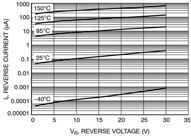
**Figure 3. Leakage Current**
