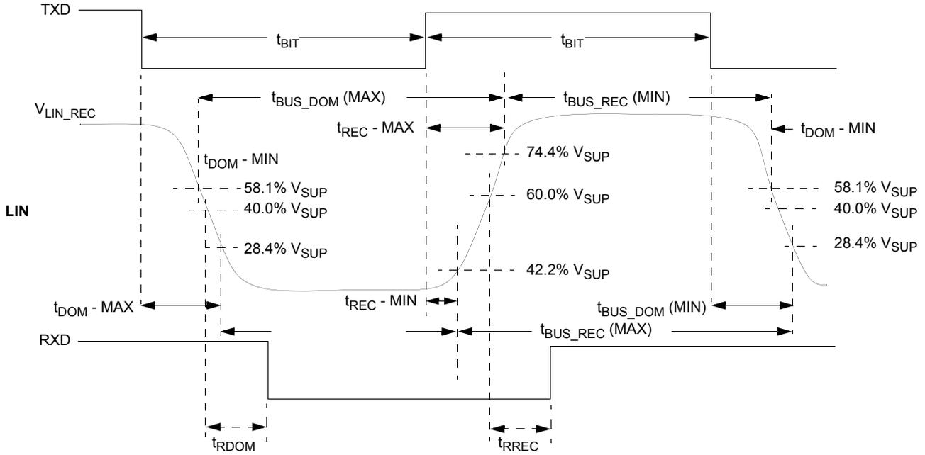
Figure 30. LIN Timing Measurements for Normal Slew Rate
