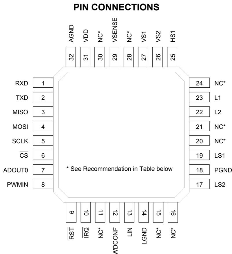
Figure 3. 33911 Pin Connections
