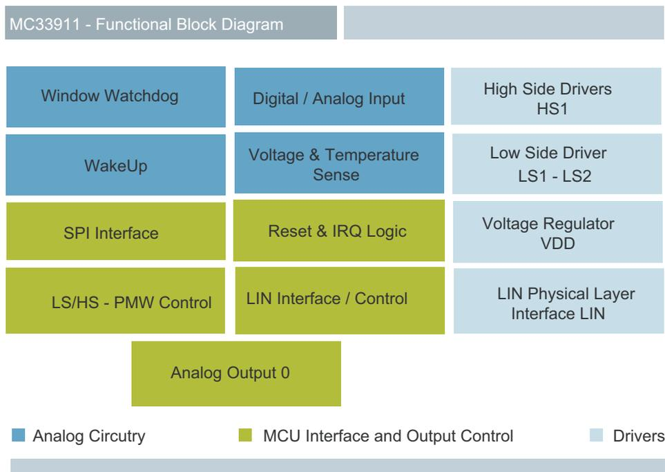
**Figure 37. Functional Internal Block Diagram****ANALOG CIRCUITRY**
