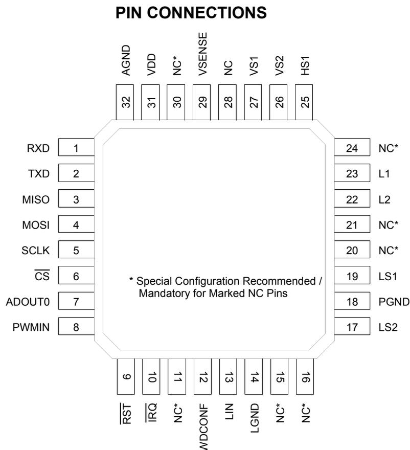
Figure 26. 33911 Pin Connections
