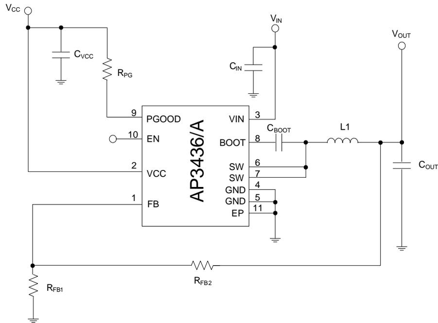
Note 4: When using a single power supply for V<sub>CC</sub> and V<sub>IN</sub>, a 4.7Ω resistor should be placed between them for noise isolation.
