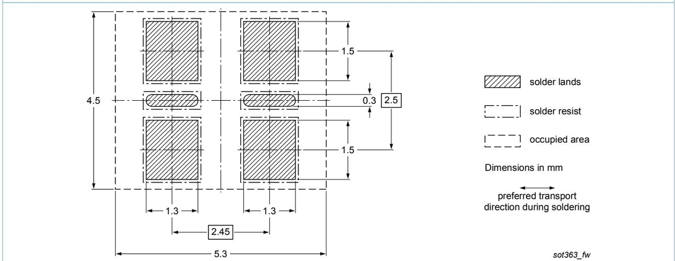
Fig. 20. Wave soldering footprint for TSSOP6 (SOT363)
