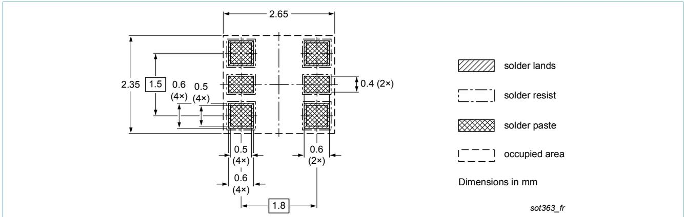
Fig. 19. Reflow soldering footprint for TSSOP6 (SOT363)
