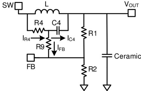
**Figure 7: Simplified PWM-Mode Circuit with External Ramp Compensation**
