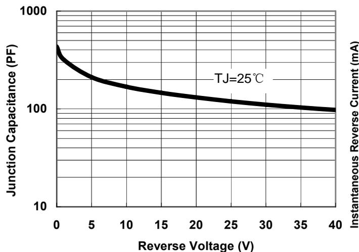
Fig.1-Typical Junction Capacitance
