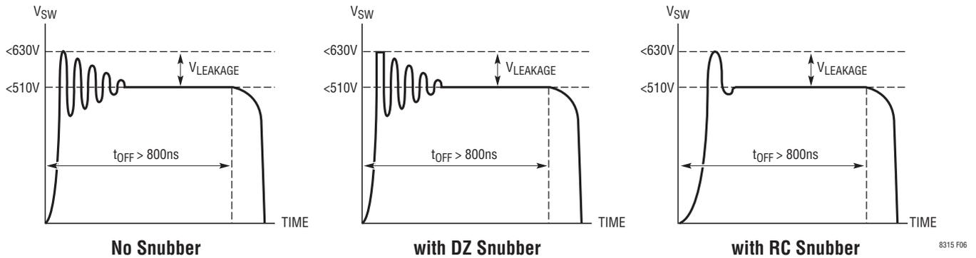
Figure 6. Maximum Voltages for SW Pin Flyback Waveform
