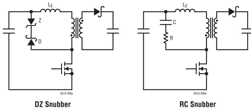
Figure 7. Snubber Circuits
