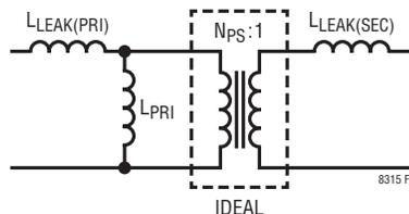
**Figure 5. Transformer Model**
