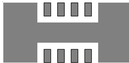
(e) Copper Area =  $70 \text{ mm}^2$ ,  $\theta_{JA} = 49^\circ\text{C/W}$
