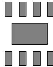
(b) Copper Area =  $10 \text{ mm}^2$ ,  $\theta_{JA} = 64^\circ\text{C/W}$
