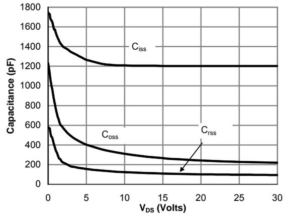
**Figure 8: Capacitance Characteristics**
