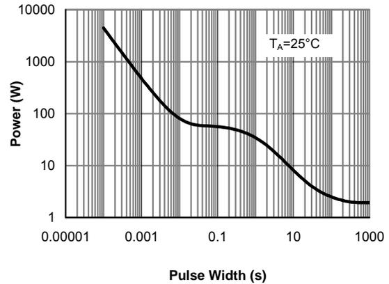
Figure 15: Single Pulse Power Rating Junction-to-Ambient (Note H)
