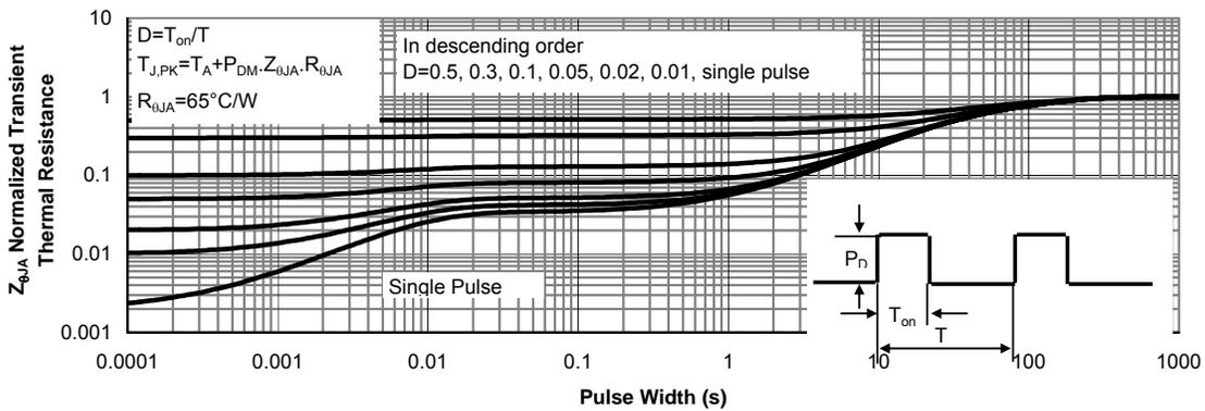
Figure 16: Normalized Maximum Transient Thermal Impedance (Note H)
