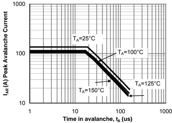
Figure 12: Single Pulse Avalanche capability (Note C)
