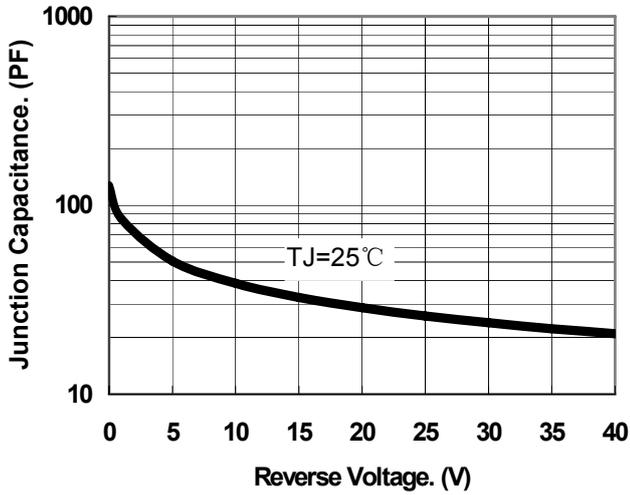
Fig.1-Typical Junction Capacitance
