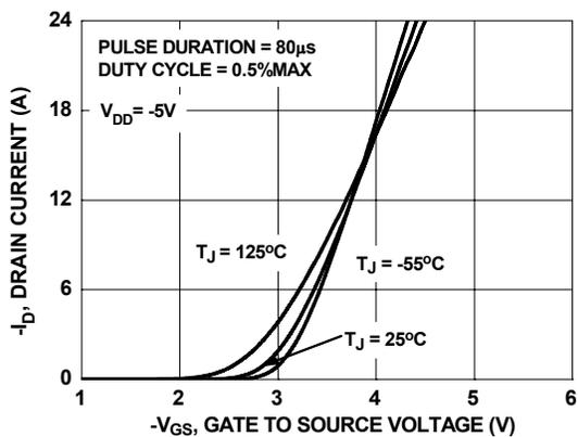
Figure 5. Transfer Characteristics
