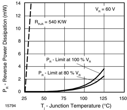
Fig. 1 - Max. Reverse Power Dissipation vs. Junction Temperature
