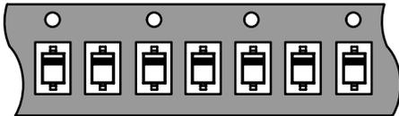
"T5" Cathode Lead Toward Sprocket Hole (8k Reel)
