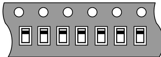
Die orientation in tape with pads down
