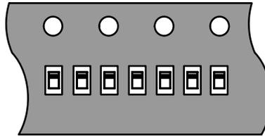
T5 – Cathode Band Toward Sprocket Hole (15k Reel)
