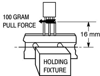
The component shall not pull free with a 300 gram load applied to the leads for  $3 \pm 1$  second.
