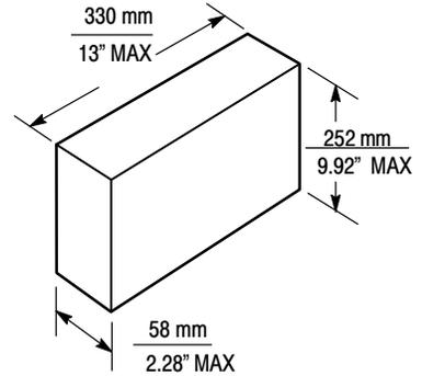
**Figure 47. Fan Fold Box Dimensions**
