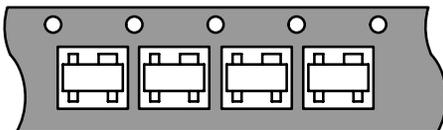
"T2" Wide Lead Tape Toward Sprocket Hole (3k Reel)
