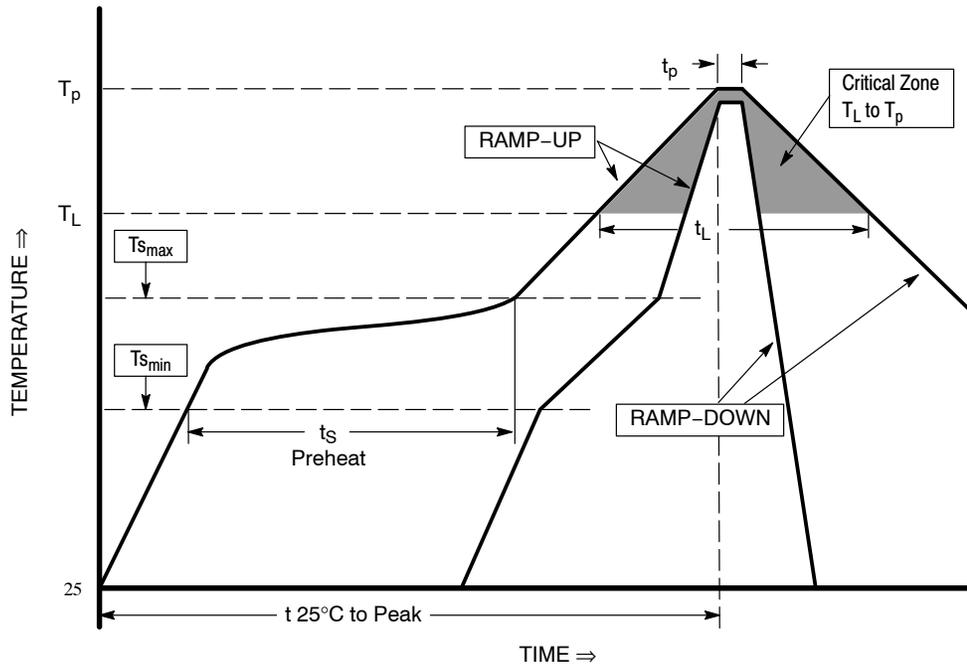
Figure 62. Typical Pb-Free Solder Heating Profile
