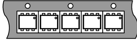
"T5" Pin One Toward Sprocket Hole (8k Reel)
