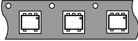
"T1" Pin One Toward Sprocket Hole (4k Reel)
