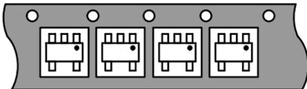
"T2" Pin One Toward Sprocket Hole (3k Reel)
