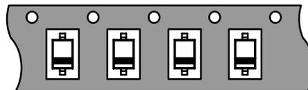
"T2" Cathode Lead Opposing Sprocket Hole (3k Reel)
