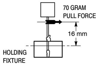
The component shall not pull free with a 70 gram load applied to the leads for  $3 \pm 1$  second.
