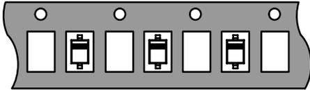
"T1" Cathode Lead Toward Sprocket Hole (3k Reel)
