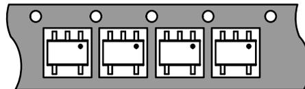
"T1" Pin One Toward Sprocket Hole (3k Reel)
