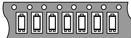
"T5" Single Lead Toward Sprocket Hole (8k Reel)
