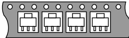
"T1" Single Lead Toward Sprocket Hole (1k Reel)
