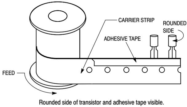
Rounded side of transistor and adhesive tape visible.
