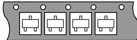
"T1" Single Lead Toward Sprocket Hole (3k Reel)
