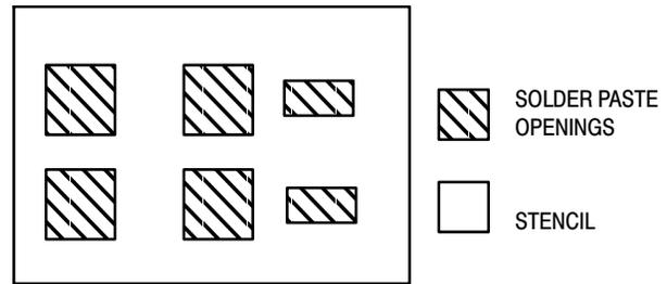
Figure 60. Typical Stencil for DPAK and D<sup>2</sup>PAK Packages
