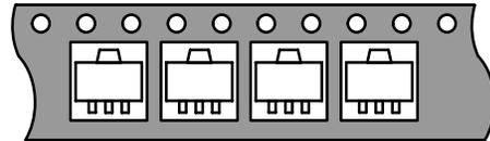
"T1" Single Lead Toward Sprocket Hole (1k Reel)
