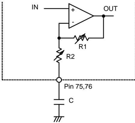
$$f_c = \frac{1}{2\pi R_2 C} \quad (\text{Hz})$$
