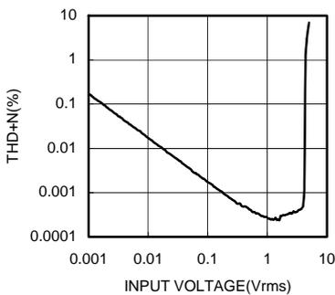
Fig.17 REC Total Harmonic Distortion - Input Voltage
