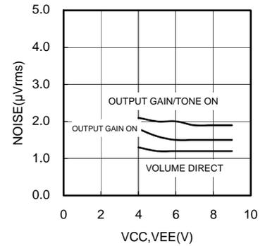
Fig.13 Output Noise Voltage - Power Supply Voltage
