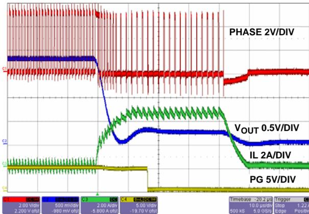
FIGURE 32. OUTPUT SHORT-CIRCUIT
