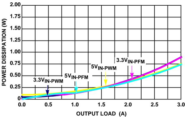
FIGURE 7. POWER DISSIPATION vs LOAD (1MHz,  $V_{OUT} = 1.8\text{V}$ )
