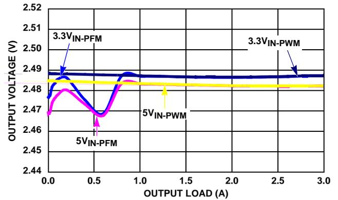
FIGURE 12.  $V_{OUT}$  REGULATION vs LOAD (1MHz,  $V_{OUT} = 2.5\text{V}$ )
