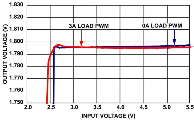
FIGURE 14. OUTPUT VOLTAGE REGULATION vs VIN (PWM  $V_{OUT} = 1.8$ )
