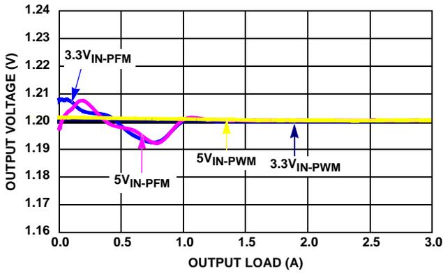
FIGURE 9.  $V_{OUT}$  REGULATION vs LOAD (1MHz,  $V_{OUT} = 1.2\text{V}$ )
