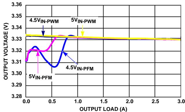
FIGURE 13.  $V_{OUT}$  REGULATION vs LOAD (1MHz,  $V_{OUT} = 3.3\text{V}$ )
