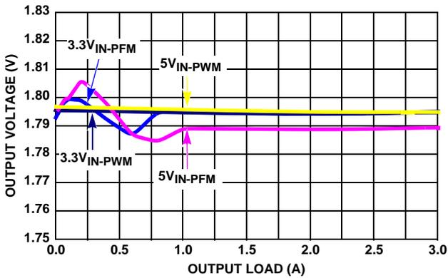
FIGURE 11.  $V_{OUT}$  REGULATION vs LOAD (1MHz,  $V_{OUT} = 1.8\text{V}$ )
