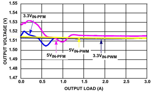
FIGURE 10.  $V_{OUT}$  REGULATION vs LOAD (1MHz,  $V_{OUT} = 1.5\text{V}$ )
