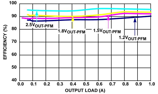
FIGURE 4. EFFICIENCY vs LOAD (1MHz 3.3  $V_{IN}$  PFM)
