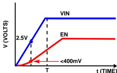
FIGURE 38. CIRCUIT IMPLEMENTATION WITH  $V_{IN}$  SLEW RATE
