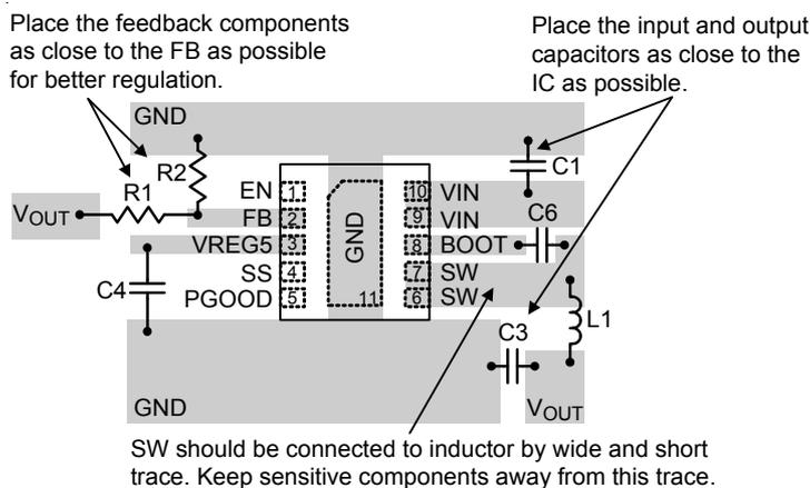
Figure 8. PCB Layout Guide for WDFN-10L 3x3 Package
