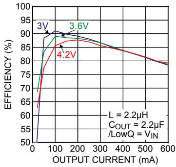
**DC/DC 1.8V<sub>OUT</sub> Efficiency**
