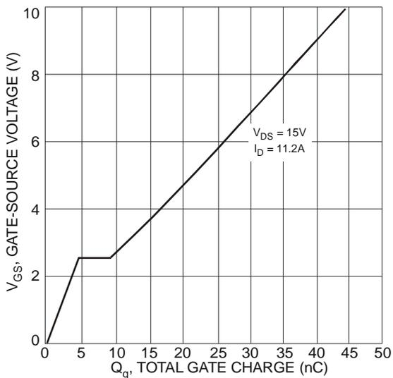
Fig. 14 Gate-Charge Characteristics
