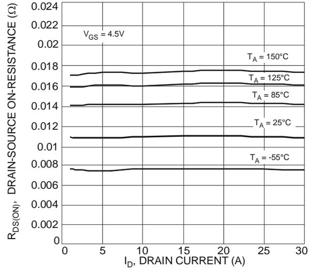
Fig. 7 Typical On-Resistance vs. Drain Current and Temperature
