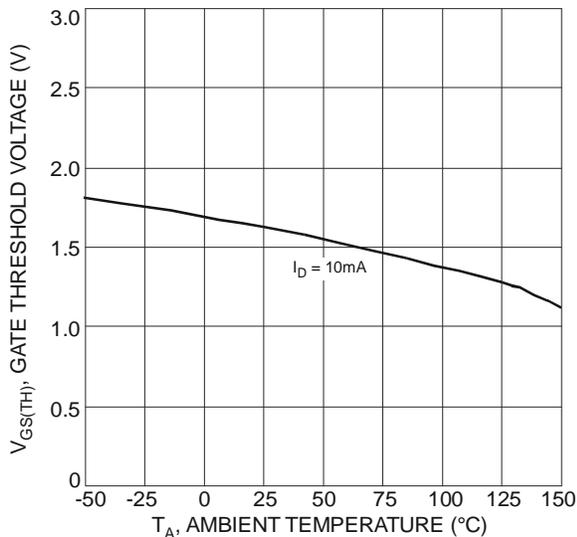
Fig. 10 Gate Threshold Variation vs. Ambient Temperature
