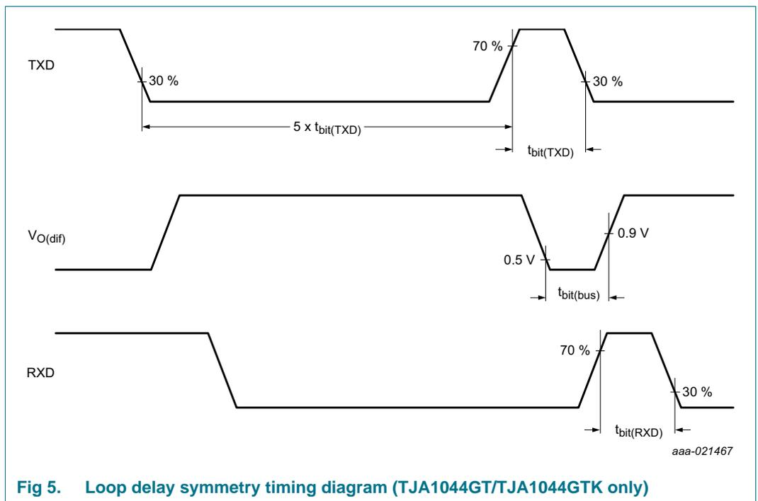
Fig 5. Loop delay symmetry timing diagram (TJA1044GT/TJA1044GTK only)
