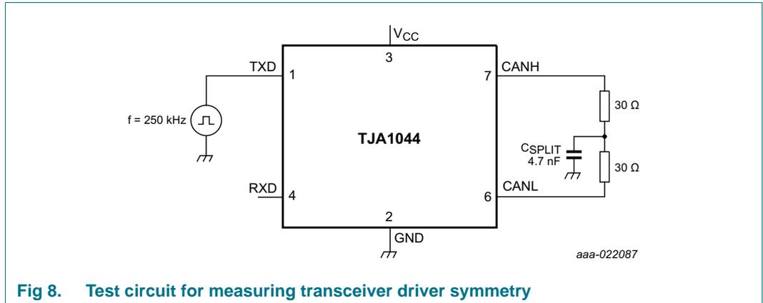
Fig 8. Test circuit for measuring transceiver driver symmetry
