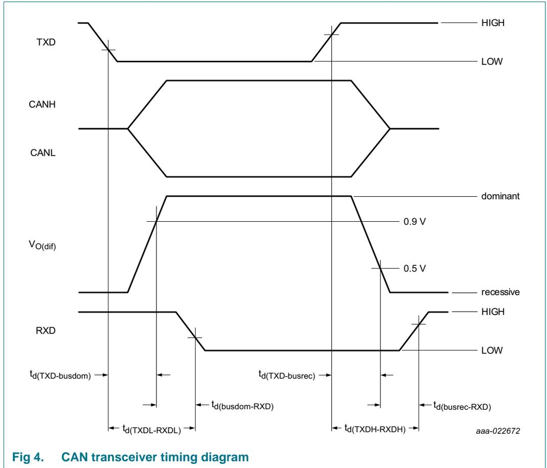
Fig 4. CAN transceiver timing diagram
