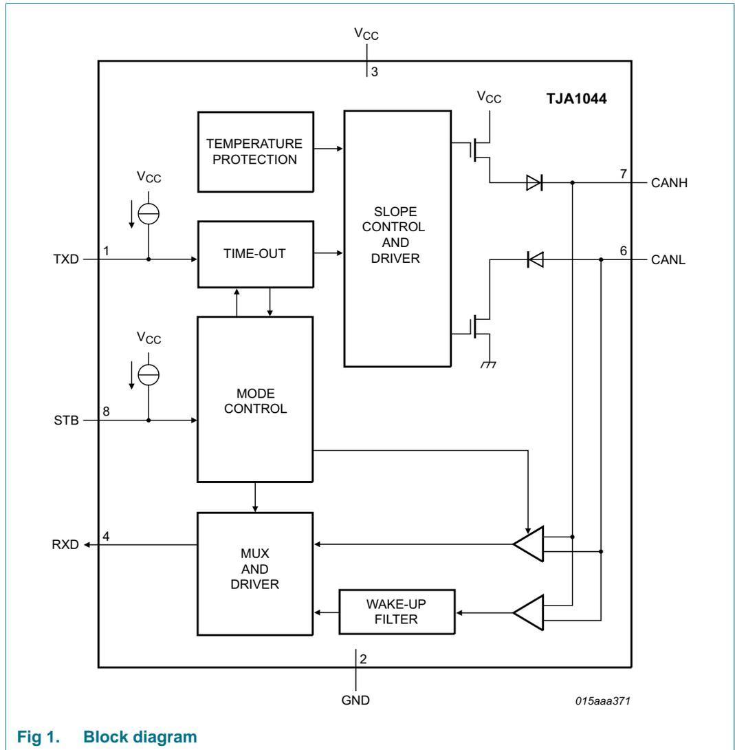
Fig 1. Block diagram
