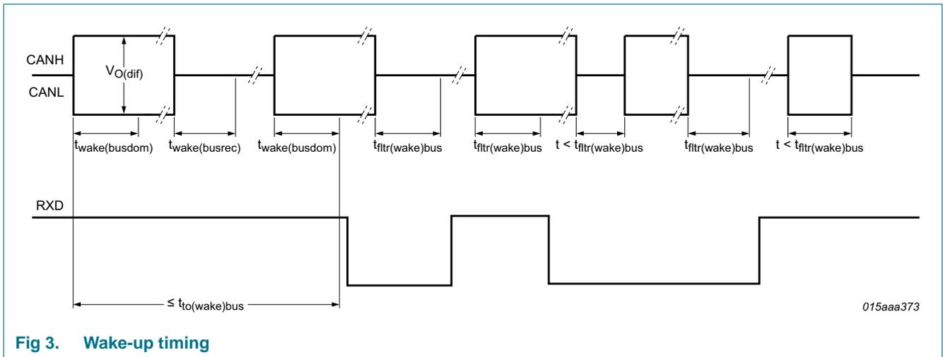
Fig 3. Wake-up timing
