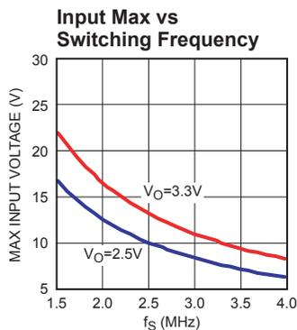
**Figure 2—Recommended Input vs.  $f_s$**
