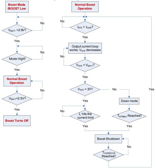
Figure 6: Operation Flow Chart in Boost Mode
