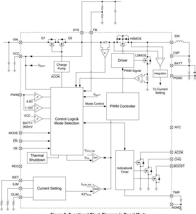
Figure 2: Functional Block Diagram in Boost Mode
