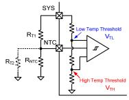
**Figure 14: NTC Function Block**
