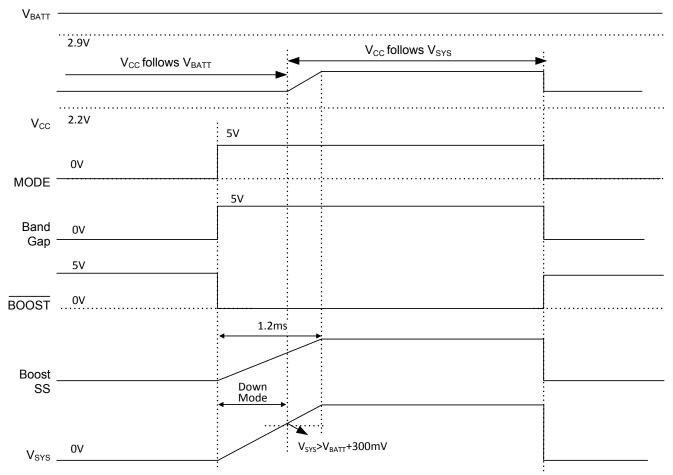
Figure 10: Mode Start-Up Time Flow in Boost Mode
