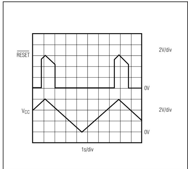
Figure 4. Typical MAX700/MAX701/MAX702 RESET Output vs. VCC
