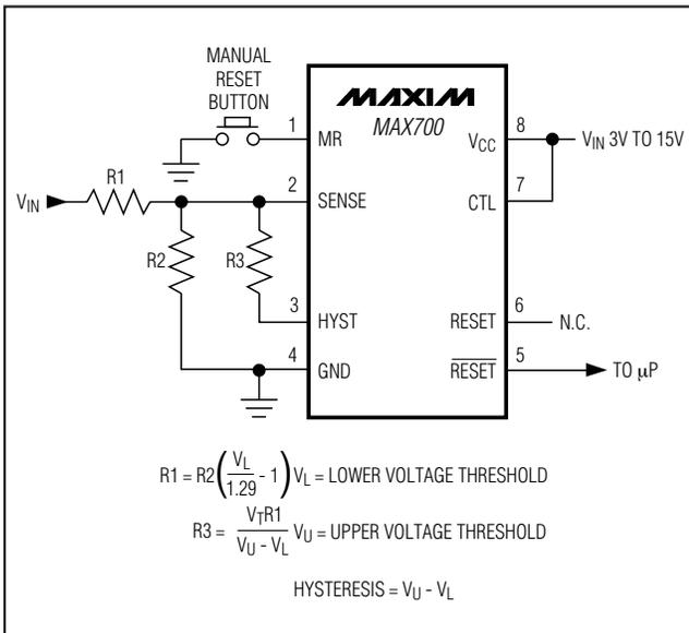
Figure 3. MAX700 Connected for External Senses and Hysteresis
