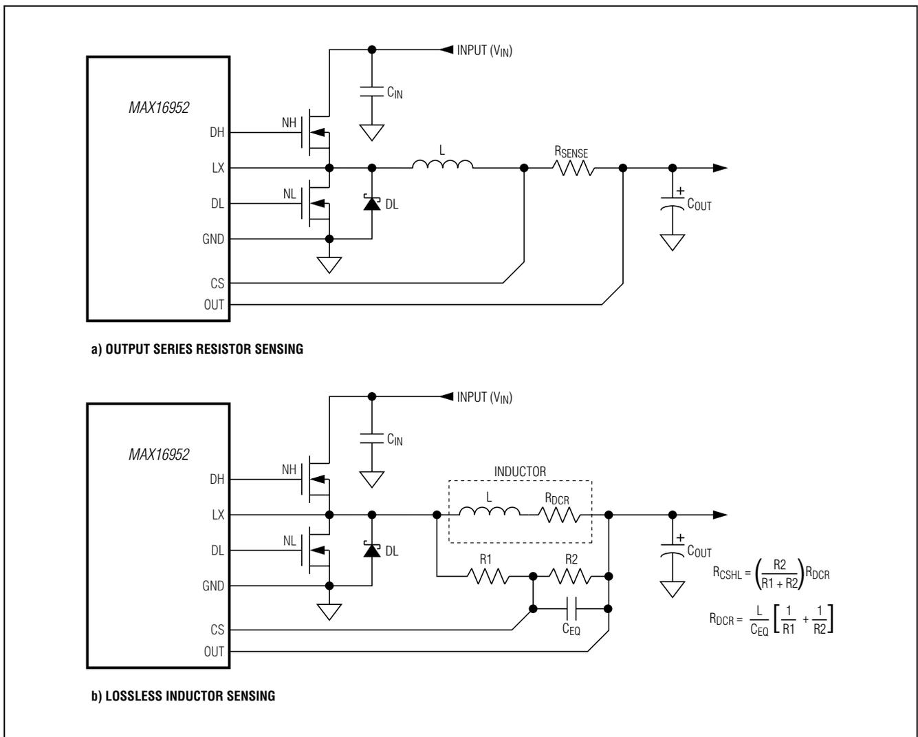
Figure 4. Current-Sense Configurations
