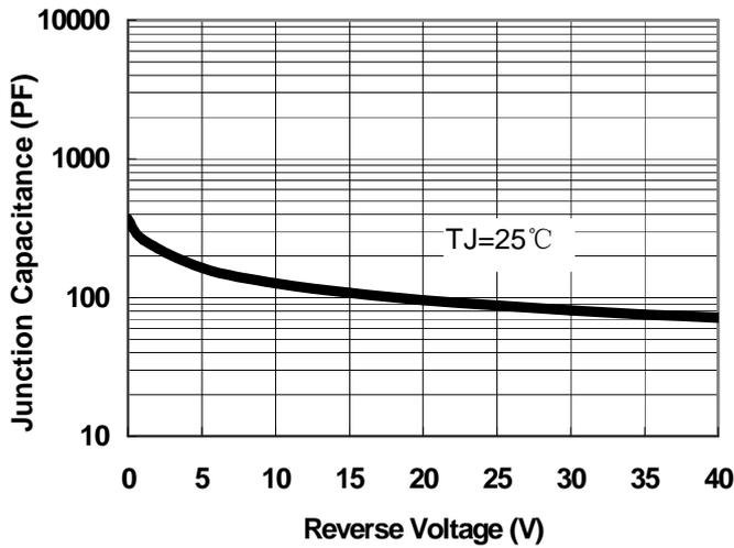
Fig.1-Typical Junction Capacitance
