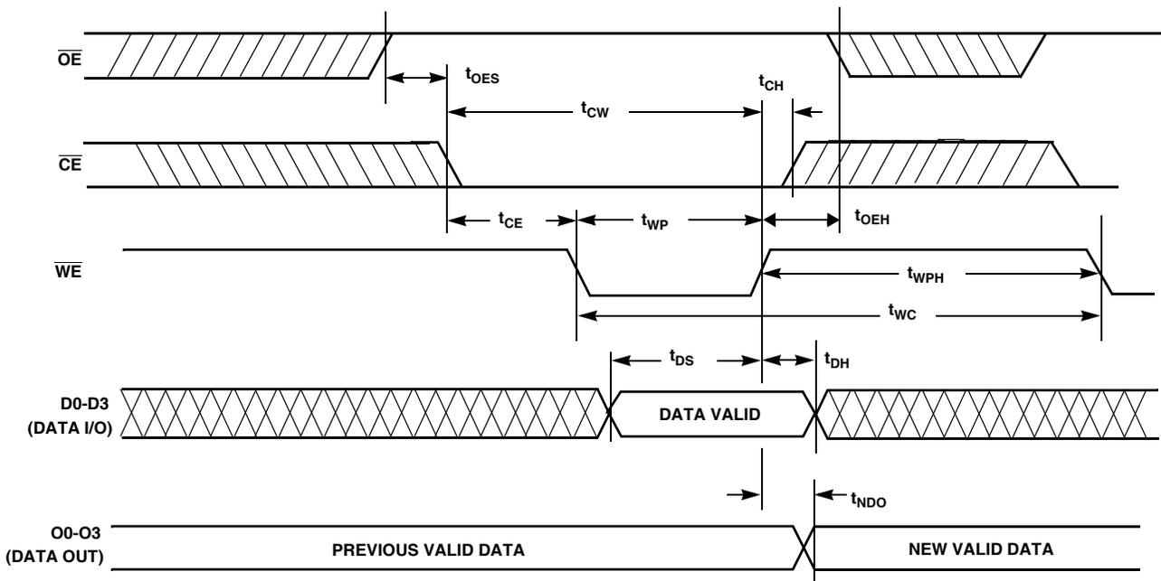
**NOVRAM  $\overline{CE}$  Controlled Write Cycle**
