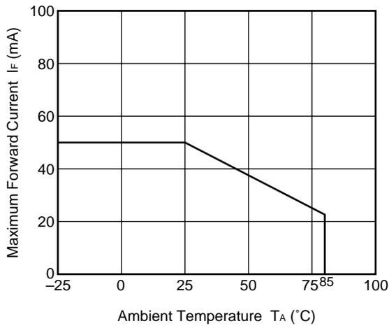
**MAXIMUM LOAD CURRENT vs. AMBIENT TEMPERATURE**
