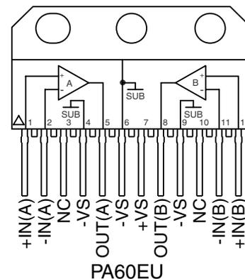
**FIGURE 3.** External connections
