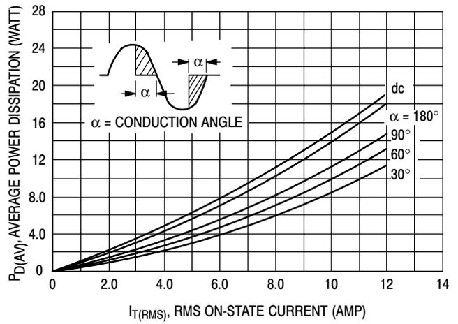
Figure 2. Power Dissipation
