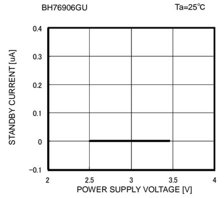
Fig. 18 Standby Circuit Current vs Supply Voltage
