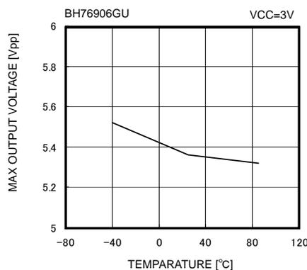
Fig. 37 Max. Output Level vs Ambient Temperature
