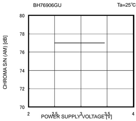
Fig. 49 C AM S/N vs Supply Voltage
