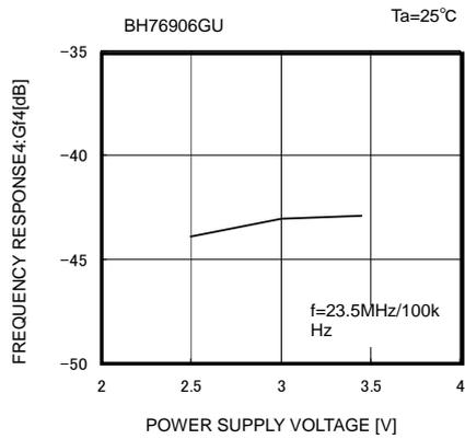
Fig. 34 Frequency Characteristic 4 vs Supply Voltage
