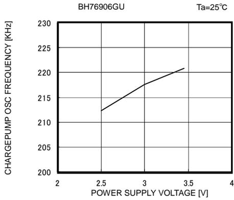
Fig. 39 Charge Pump Oscillation Frequency vs Supply Voltage
