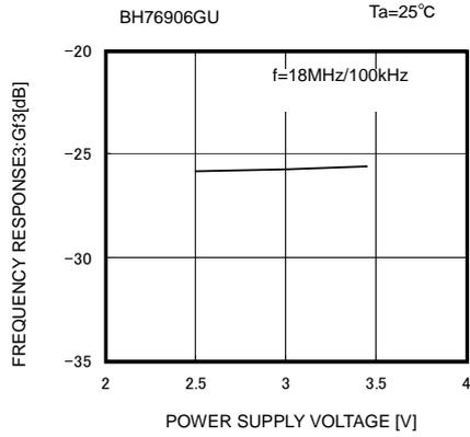
Fig. 32 Frequency Characteristic 3 vs Supply Voltage
