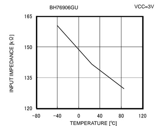
Fig. 54 Input Impedance vs Ambient Temperature
