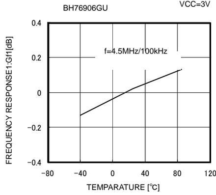
Fig. 29 Frequency Characteristic 1 vs Ambient Temperature
