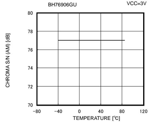
Fig. 50 C AM S/N vs Ambient Temperature
