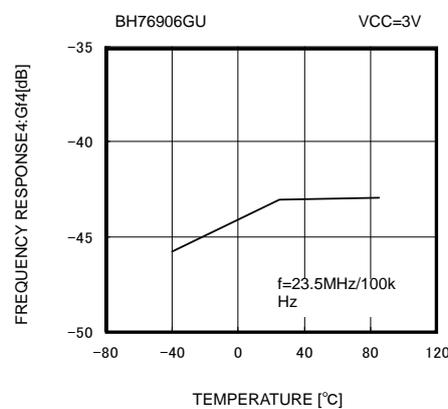
Fig. 35 Frequency Characteristic 4 vs Ambient Temperature
