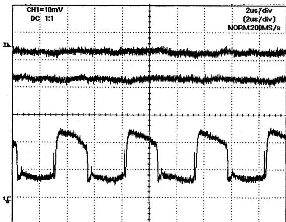
Waveform of current between power supply and capacitor (A)
