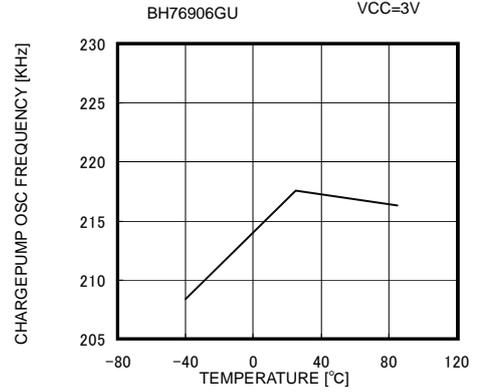
Fig. 40 Charge Pump Oscillation Frequency vs Ambient Temperature
