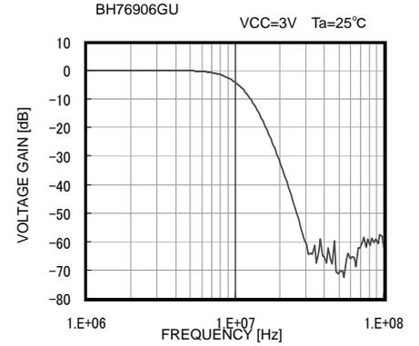
Fig. 24 Frequency Characteristic
