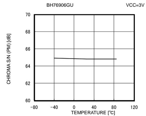
Fig. 52 C PM S/N vs Ambient Temperature
