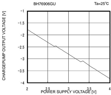
Fig. 41 Charge Pump Output Voltage vs Supply Voltage
