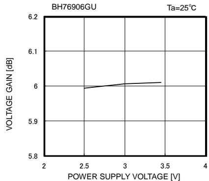
Fig. 26 Voltage Gain vs Supply Voltage
