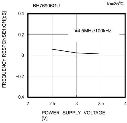
Fig. 28 Frequency Characteristic 1 vs Supply Voltage
