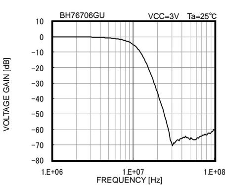
Fig. 25 Frequency Characteristic
