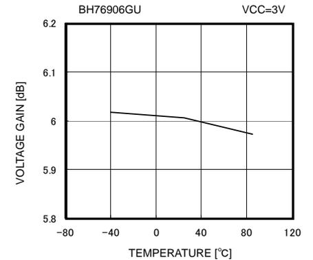
Fig. 27 Voltage Gain vs Ambient Temperature
