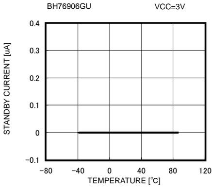
Fig. 19 Standby Circuit Current vs Ambient Temperature
