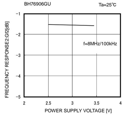
Fig. 30 Frequency Characteristic 2 vs Supply Voltage
