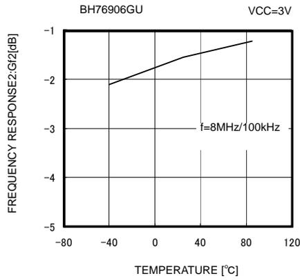
Fig. 31 Frequency Characteristic 2 vs Ambient Temperature
