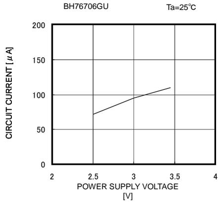
Fig. 20 GND Mode Circuit Current vs Supply Voltage
