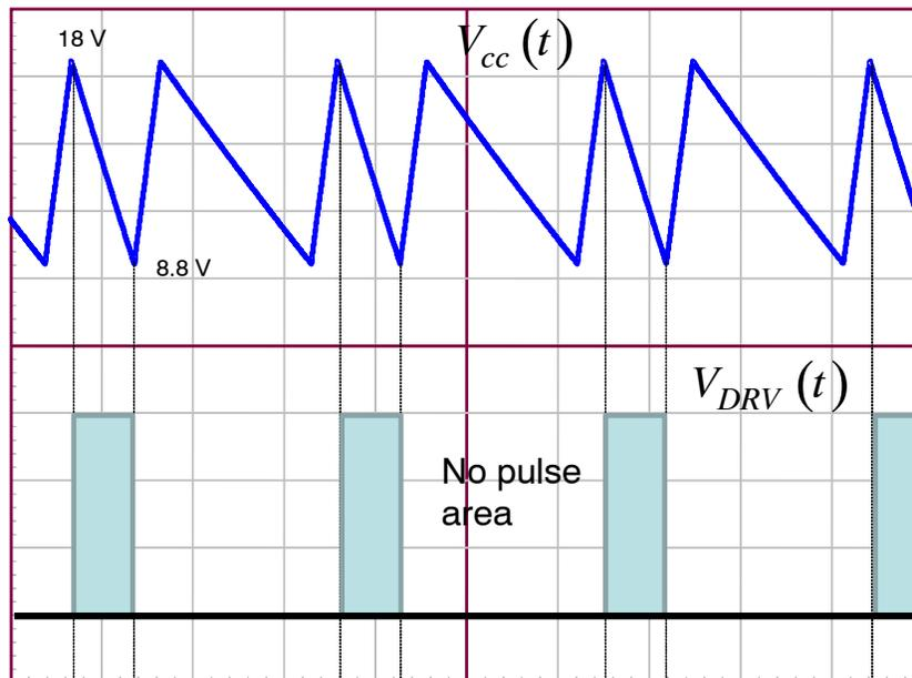
Figure 6. An Auto-Recovery Hiccup Mode is Entered in Case a Faulty Event Longer than 100 ms is Acknowledged by the Switcher
