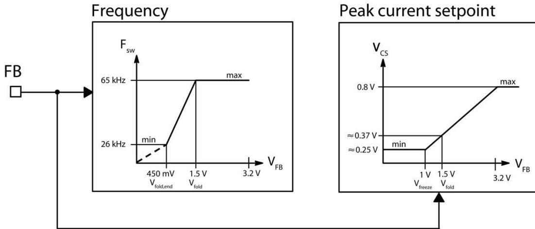
Figure 5. By Observing the Voltage on the Feedback Pin, the Switcher Reduces its Switching Frequency for an Improved Performance at Light Load
