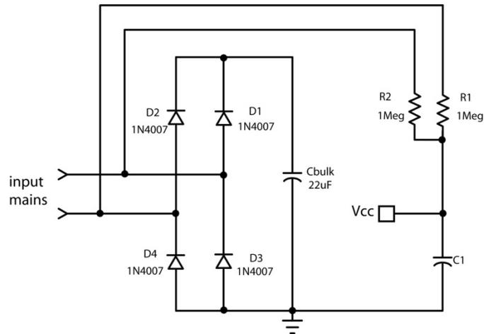
**Figure 4. The Full-Wave Connection Ensures Latch Current Continuity as well as a X2-Discharge Path**
