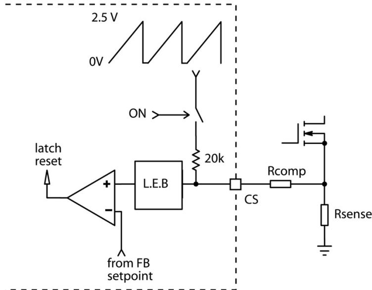
**Figure 7. Inserting a Resistor in Series with the Current Sense Information Brings Slope Compensation and Stabilizes the Converter in CCM Operation**
