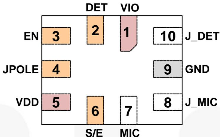
Figure 2. 10-Lead UMLP Pin Assignment (Through View)
